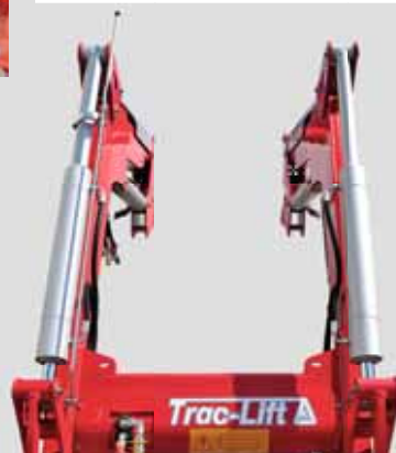
Protected hydraulic system is placed inside the loader arms and inside front bracing strut. The bracing strut also increases solidity of the loader.
