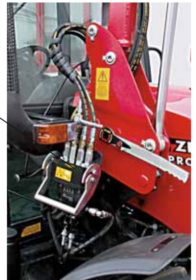
Unique connecting system allows quick, solid and safe connection of the loader to the tractor.
